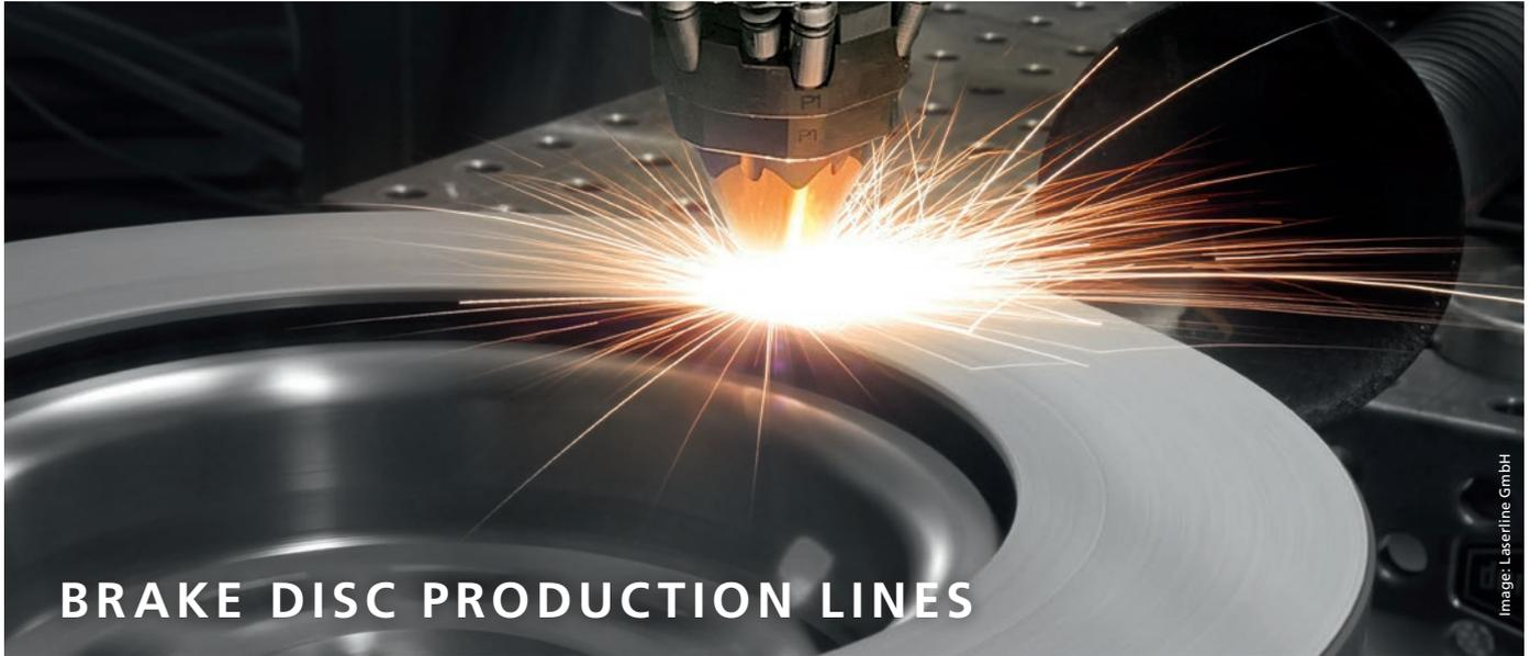
The rising amount of passenger cars worldwide and continuously increasing emission of fine dust pollution channel the focus on the fine dust emission of the vehicles' brake systems. They constitute about 15 % of the total emissions of road traffic. Due to laser cladding the fine dust of brake discs can be reduced by 90 %.
