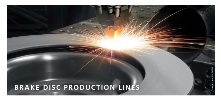
The rising amount of passenger cars worldwide and continuously increasing emission of fine dust pollution channel the focus on the fine dust emission of the vehicles' brake systems. They constitute about 15% of the total emissions of road traffic. Due to laser cladding the fine dust of brake discs can be reduced by 90%.
